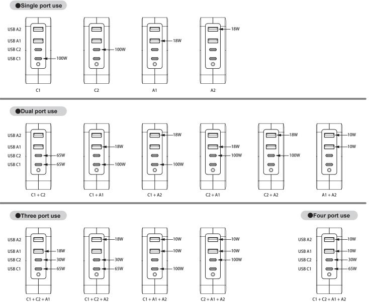
\* When using 3 or more ports with 2 USB-C ports in use, the maximum USB C1 is 65W and the maximum USB C2 is 30W.
