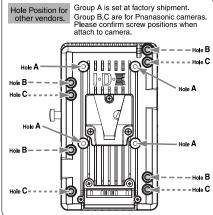
Please check the input voltage of the camera or other equipment prior to selecting the correct P-V Plate for your application.
