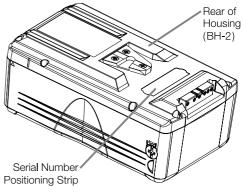
6 Align the Slide Cover to the Open/Close Position Adjusting Mark and close by sliding it upwards. Turn the Slide Cover Lock to the "Lock" position.
