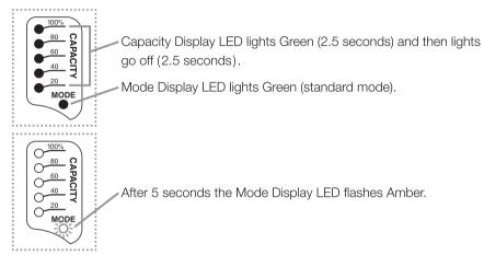
With the flashing active, tap the Capacity Display Button once to initiate the SB Mode.
