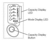
For the error contents, refer "Error Display" and "Error Code" section. When fully charging the Capacity Display LED shows 100% and the Mode Display LED lights Green.
